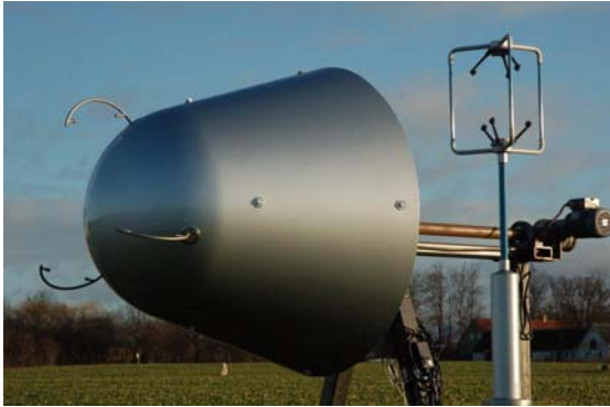
Figure 11 The spinner anemometer in comparison to a 3D sonic anemometer
