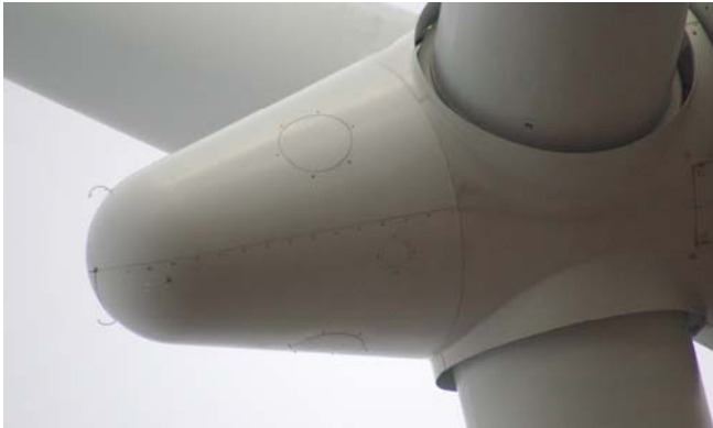
Figure 16 The three 1D sonic wind sensors mounted on the 3,6MW wind turbine spinner at the Risø Høvsøre test station
