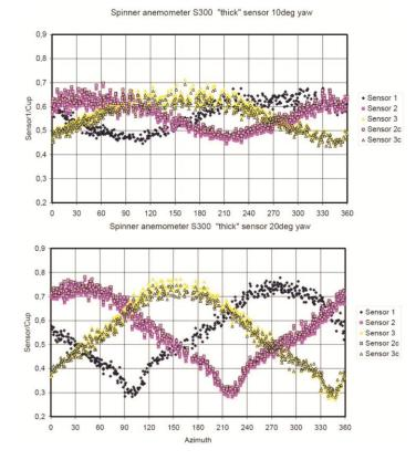
Wind speeds measured by Spinner SONIC (sensor 1, 2, 3) during consecutive rotations of the spinner at a yaw angle of 10° (upper) and 20° (lower) relative to non-rotating reference measurement (sensor 2c, 3c).
