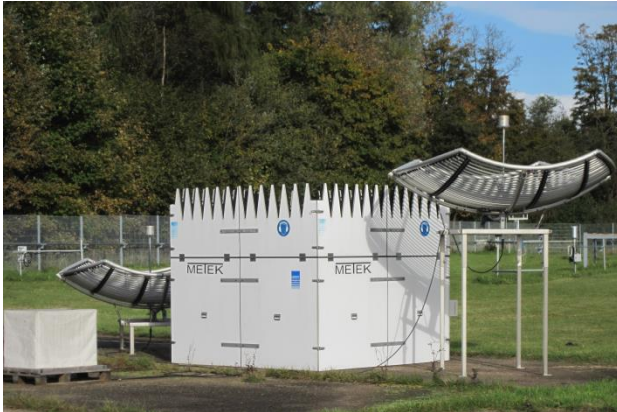
SODAR PCS.2000-64 with 1290 MHz RASS extension (antenna Ø 2.4 m)
